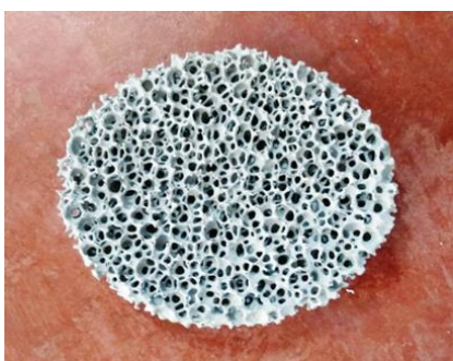
Fig. 8. Ceramic foam filter
