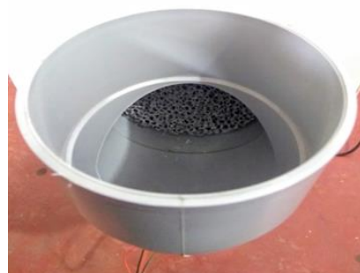
Fig. 11. Ceramic foam filter
