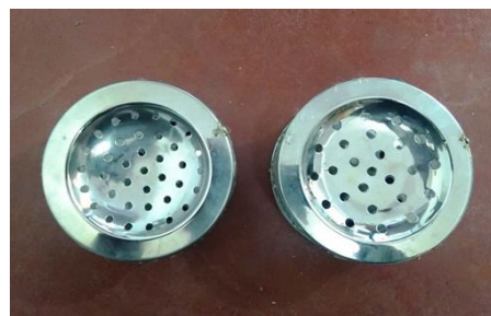
Fig. 5. Stainless steel alloy collection electrodes
