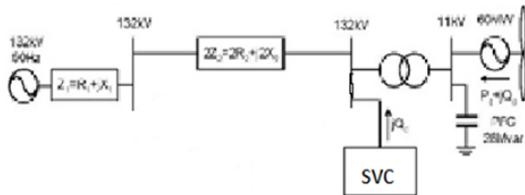
Fig. 7. Schematic diagram of simulated system
