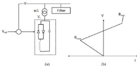
Fig. 3. Basic model and Voltage current characteristics of SVC
