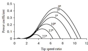
Fig. 2. Steady state characteristics between  $C_p$  and  $\lambda$  for different pitch angle ( $\beta$ )
