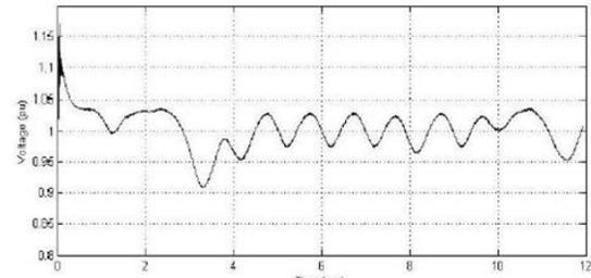
VOLTAGE FLUCTUATIONS DUE TO POWER FLUCTUATIONS (WITHOUT SVC)
