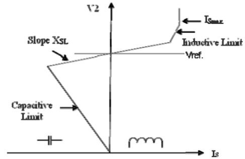
Fig. 4. SteadyState V-I Characteristic of SVC
