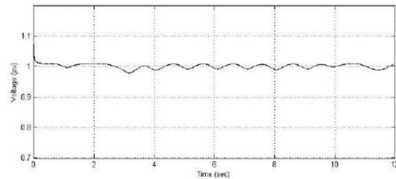
Fig. 9. Simulated results with PFC and SVC
