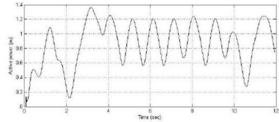
ACTIVE POWER FLUCTUATION DUE TO WIND SPEED VARIATION
