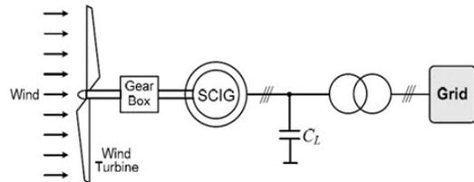
Fig. 1. Configuration of fixed speed wind turbine generator
