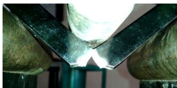
Fig. 22. Three-point bending test of coated SENTW specimen
