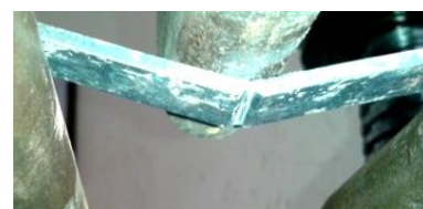
Fig. 27. Three-point bending test carburized SENWT specimen.
