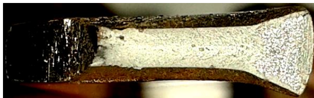
Fig. 23. Fractured surface of coated SENTW specimen due to three-point bending.
