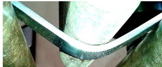
Fig. 25. Three-point bending test coated then heat treated NBT specimen.
