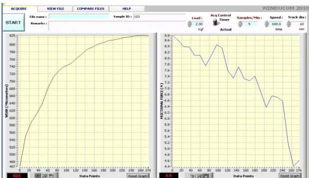
Fig. 18. Wear value for sample 04
