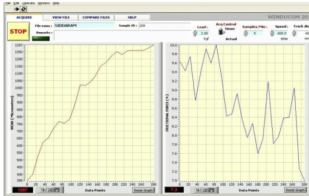
Fig. 23. Wear value for sample 09
