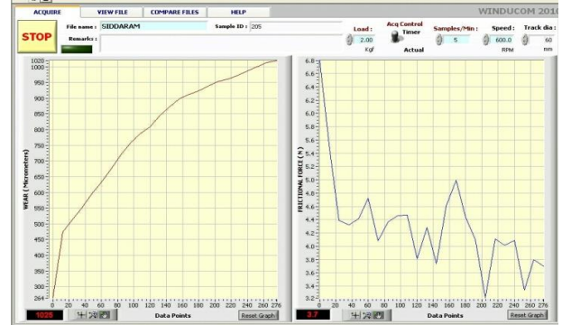
Fig. 19. Wear value for sample 05
