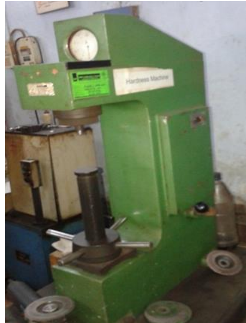
Fig. 7. Brinell Hardness Tester
