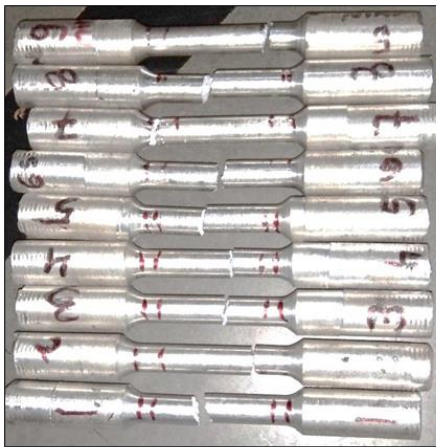
Fig. 11. Tensile Samples after testing
