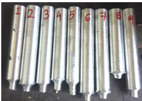
Fig. 12. Hardness Samples before testing
