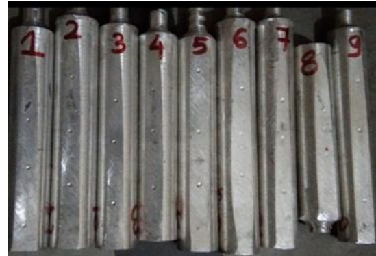
Fig. 13. Hardness Samples after testing
