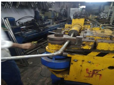
Fig. 7. Bending operation on CNC
