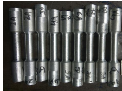
Fig. 10. Tensile Samples before testing
