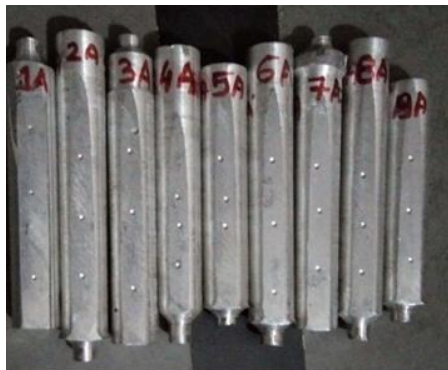
Fig. 13. Hardness Samples after testing
