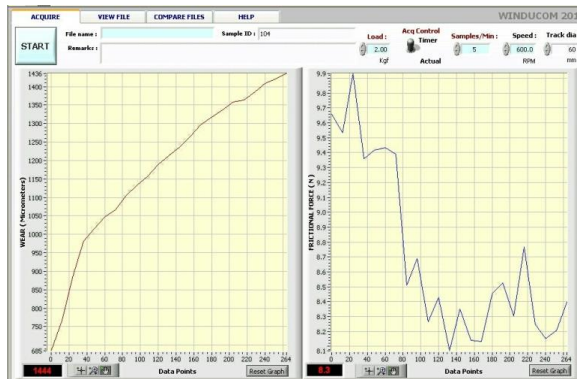
Fig. 18. Wear value for sample 04
