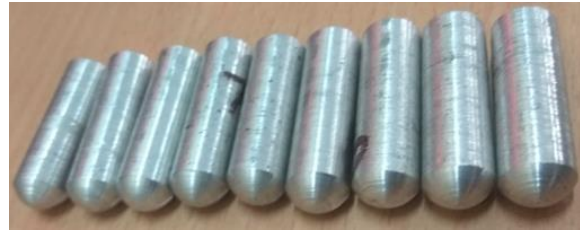
Fig. 14. Wear sample for testing
