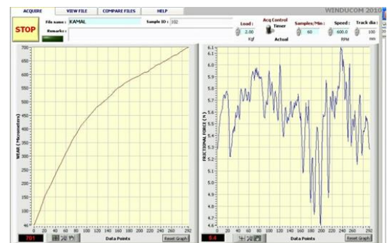
Fig. 16. Wear value for sample 02
