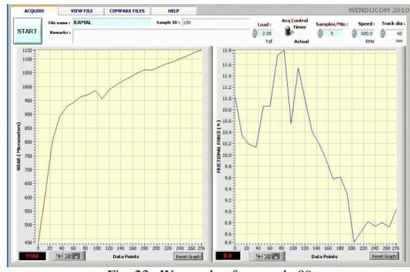
Fig. 23. Wear value for sample 09
