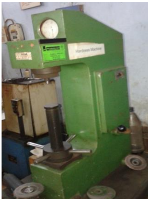
Fig. 7. Brinell Hardness Tester
