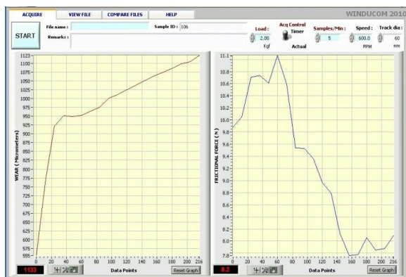
Fig. 20. Wear value for sample 06
