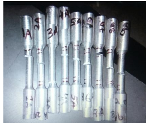
Fig. 11. Tensile Samples after testing
