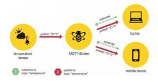
Fig. 1. MQTT protocol operation
