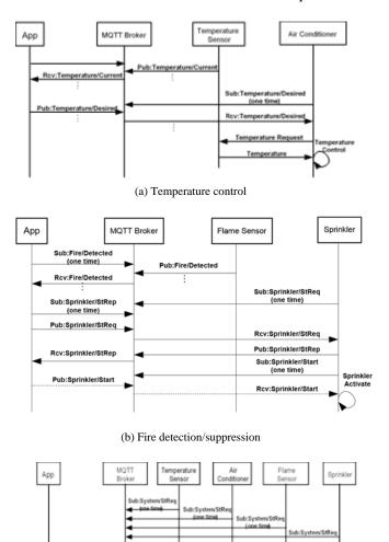
Fig. 2. IoT message exchange procedure
