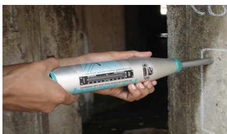
Fig. 8. Rebound hammer test
