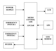
Fig. 1. Proposed method block diagram
