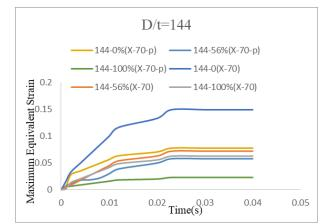
Fig. 7. Comparison of variations of X-70, D/t=144 pipe line under blast loading, with and without protective cover at different operating pressure
