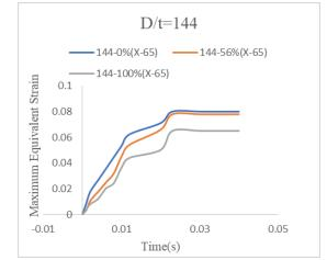
Fig. 4. Variations of X-65, D/t=144 under blast loading with protective cover and different operating pressures
