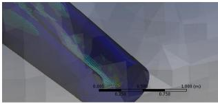
Fig. 2. Deformed shape of X-65 steel pipe at no pressure without protective cover applied
