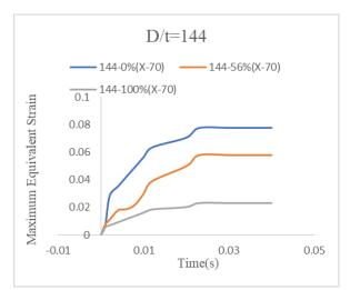
Fig. 5. Variations of X-70, D/t=144 under blast loading with protective cover and different operating pressures
