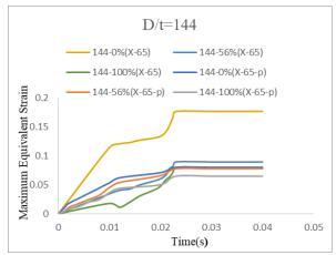
Fig. 6. Comparison of X-65 pipe line, D/t=144 under blast loading, with and without protective cover at different operating pressure (P- Protective Cover)
