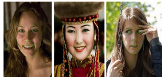
Fig. 6. Facial landmark detection using ensemble of cascaded regressions
