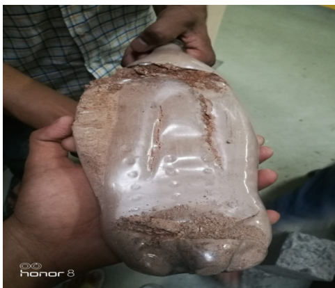
Fig. 5. Crushed bottle brick after testing
