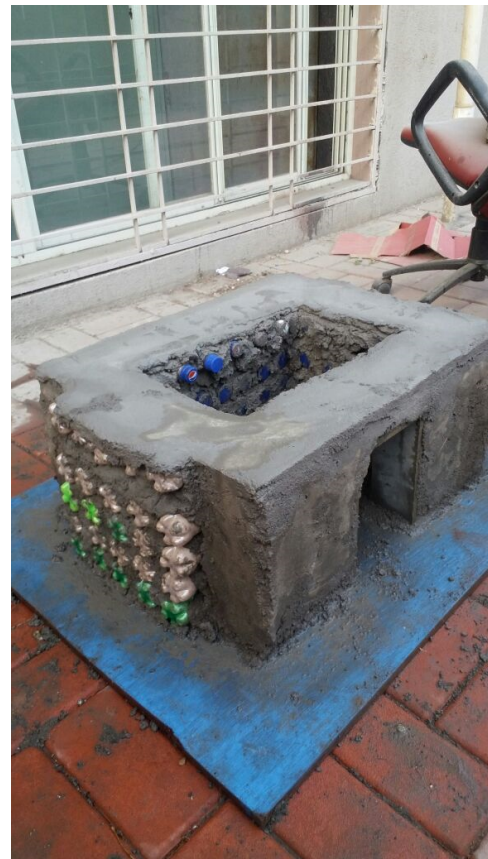
Fig. 2. Model constructed with bottle brick and cement mortar
