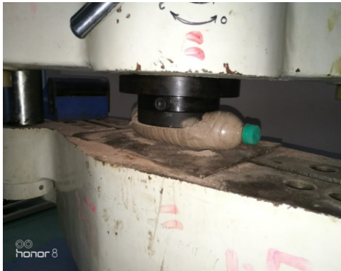
Fig. 4. Testing of bottle brick in UTM
