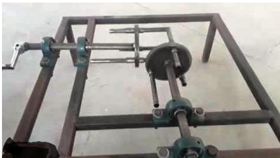
Fig. 12. Design and Fabricated Gearless Transmission Setup
